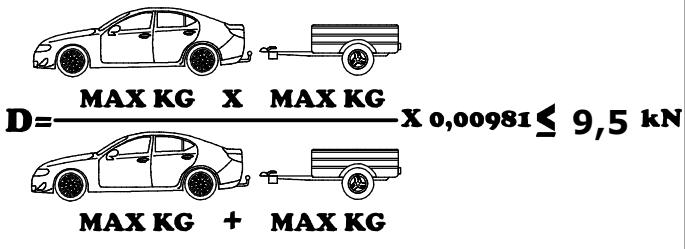
$$D = \frac{\text{MAX KG} \times \text{MAX KG}}{0,00981} \leq 9,5 \text{ kN}$$
